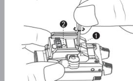
4. Position the Glock rail adapter (already installed) or Picatinny rail adapter (to be installed first) to the desired rail notch and then close the swing arm.
