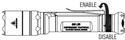
**To lock out tailcap**, rotate counterclockwise until light will not activate when pushbutton is pressed.
